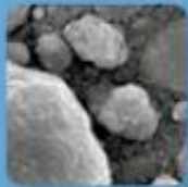
SEM Image (1 \mu\text{m} ; 20,000x magnification) Filtek Supreme XTE, 3M Espe
